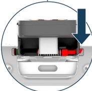
3. Align the red pin of the adapter with the notch on the case and push down into the case.
