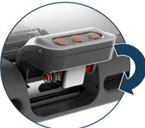
4. Flip down adapter and push to engage with port.
