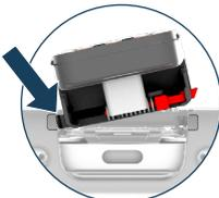
2. Holding the adapter at a 90degree angle, insert the left pin into the case.
